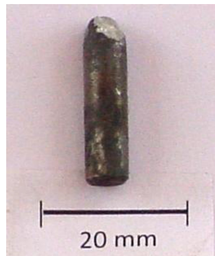
Fig. 3. Failed 7.62 mm AP projectile after ballistic impact with 5 mm thick boron carbide tile backed by Al6063 alloy.
