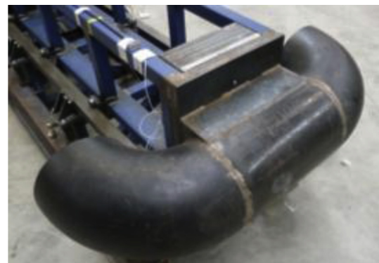
Fig. 1. The interchangeable impact head used in the experimental testing.
