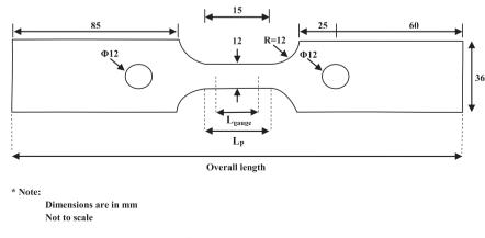
Fig. 1. Test specimen geometry.
