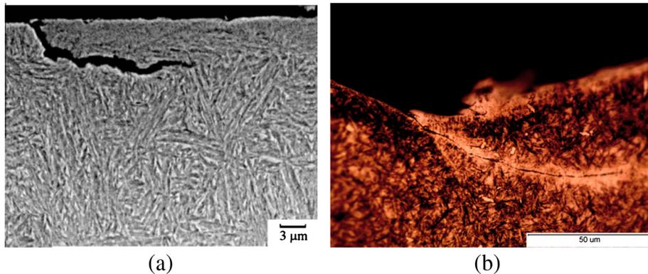
Fig. 1. Failure due to surface pitting (a) [62] as opposed to subsurface spalling (b) (note the depth of the cracks).
