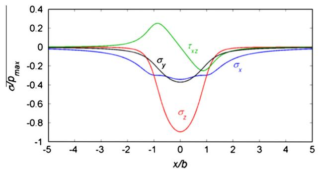
Fig. 2. Stress history for a point located at  $0.5b$  as a function of distance from the center of a moving Hertzian contact.
