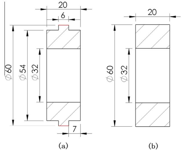
Fig. 2. The geometry sizes of the RCF specimens: (a) the tested roller with coating; and (b) the paired contact roller.
