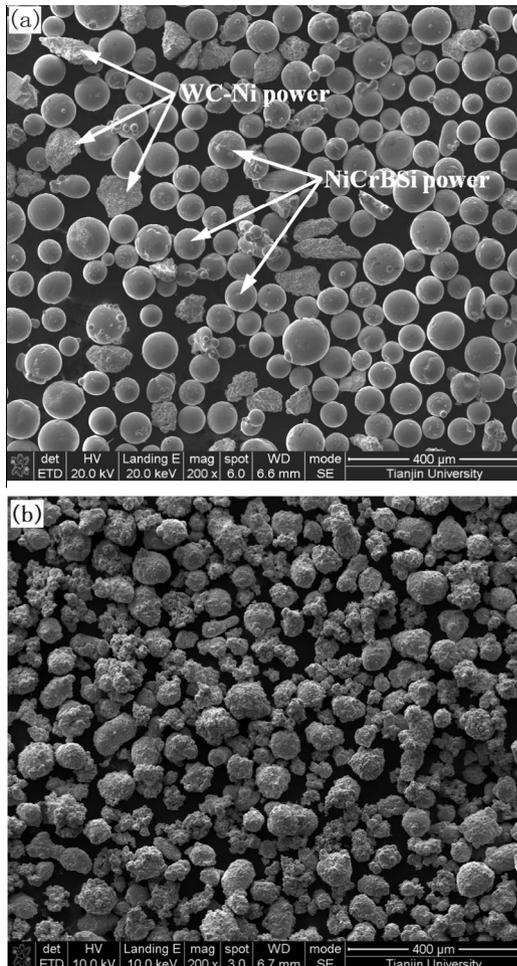
Fig. 1. Morphology of spraying powders: (a) NiCrBSi/WC–Ni composite powders; and (b) NiAl alloy powders.
