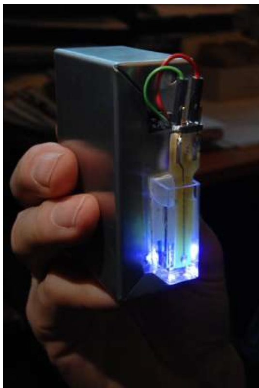
Fig. 1. Photograph of the handheld-type of PECS sensor, illuminated by a light-emitting diode. The experiments reported herein were performed on a larger scale of this setup, using a xenon strobe light as the light source, and the duration of the flash was t < 10 \mu\text{s} .
