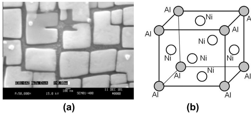
Fig. 1. (a) Typical microstructure of Ni-based superalloy single crystal PWA 1484. (b) Scheme of crystallographic cell of  $L1_2$  structure.
