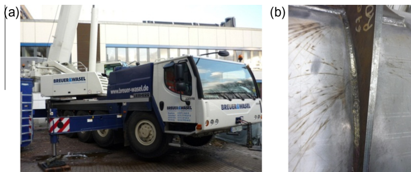
Fig. 1. Application of ultra high strength fine grained structural steels in mobile crane structures (a) and detail of a telescopic boom with welded stiffeners on a box-girder (b).
