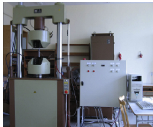
Fig. 1. UFP 400 stand for fatigue testing.
