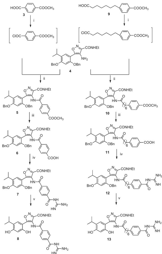
**Scheme 1.** Synthesis of guanidine bearing derivatives **8** and **13**. Reagents and conditions: (i): oxalyl chloride, DMF,  $\text{CH}_2\text{Cl}_2$ , 4 h, rt; (ii):  $\text{CH}_2\text{Cl}_2$ , TEA, 16 h, rt; (iii): MeOH, 1 N NaOH,  $\text{H}_2\text{O}$ , 24 h, 70 °C; (iv): DMF, CDI, 1 h, rt,  $\text{CH}_5\text{N}_3\text{HCl}$ , 16 h, rt; (v): 1 M  $\text{BCl}_3$ ,  $\text{CH}_2\text{Cl}_2$ , -78 °C, 1 h.
