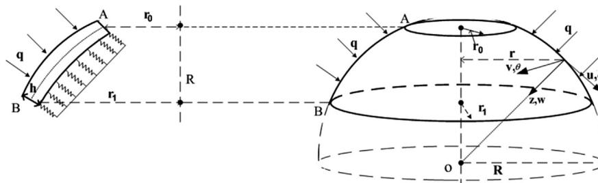
Fig. 1. Configuration of a FGM annular spherical shell.
