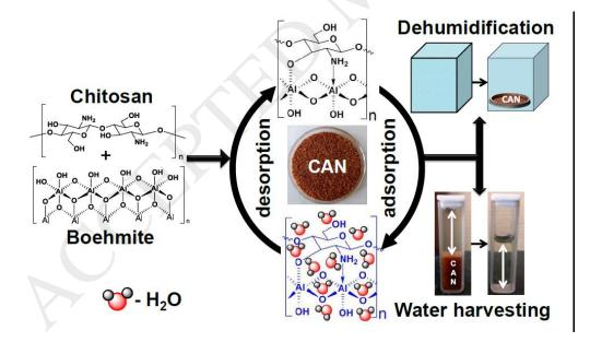
Schematic showing the formation and the ability of the composite (CAN) to dehumidify water.
