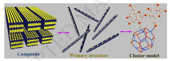
The structure-ordered cellulose/zinc oxide composite was experimentally and theoretically explored, which provide an in-depth understanding of interfacial behavior between biopolymer and semiconductor metal oxides and implications for prospective application. It is found that the electrostatic attraction drives the formation of the primary structure and the electron transfer enhances interfacial interaction. It is a dative bond per se and dominated by orbital attractions.
