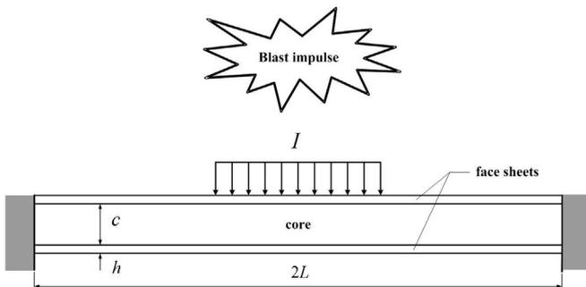
Fig. 1. Sketch of a fully clamped sandwich beam under impulsive loading over a central patch.
