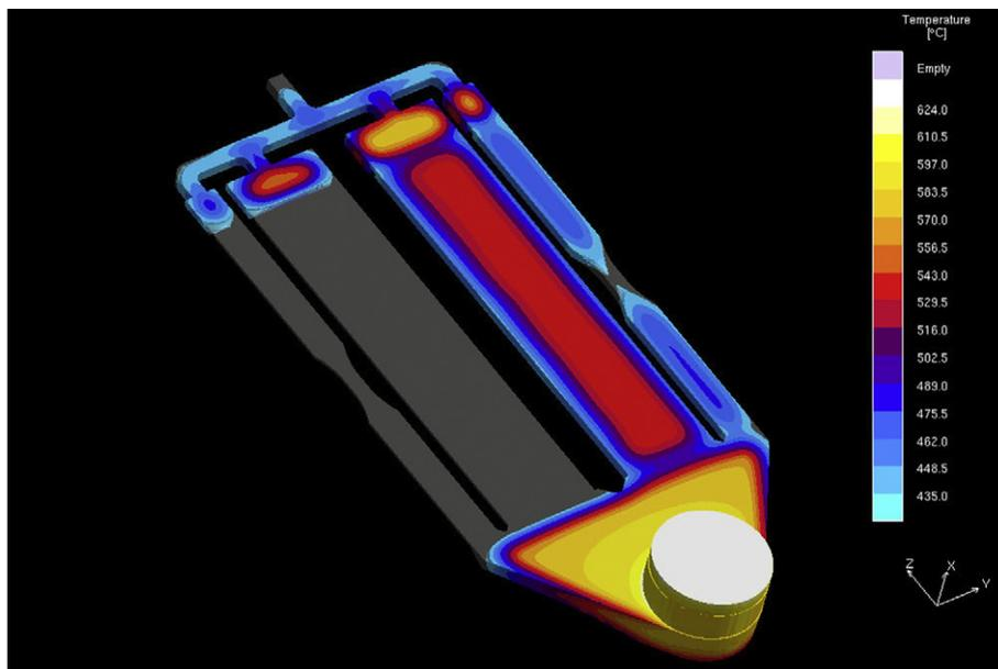
**Fig. 1.** Simulation of temperature during the solidification of the cast: In contrast to the completely solidified two specimens on the left hand with 2 mm wall thickness, the two specimens on the right with 6 mm wall thickness contain liquid parts. This means that the right hand side cannot be fed sufficiently and shrinkage porosity arises.
