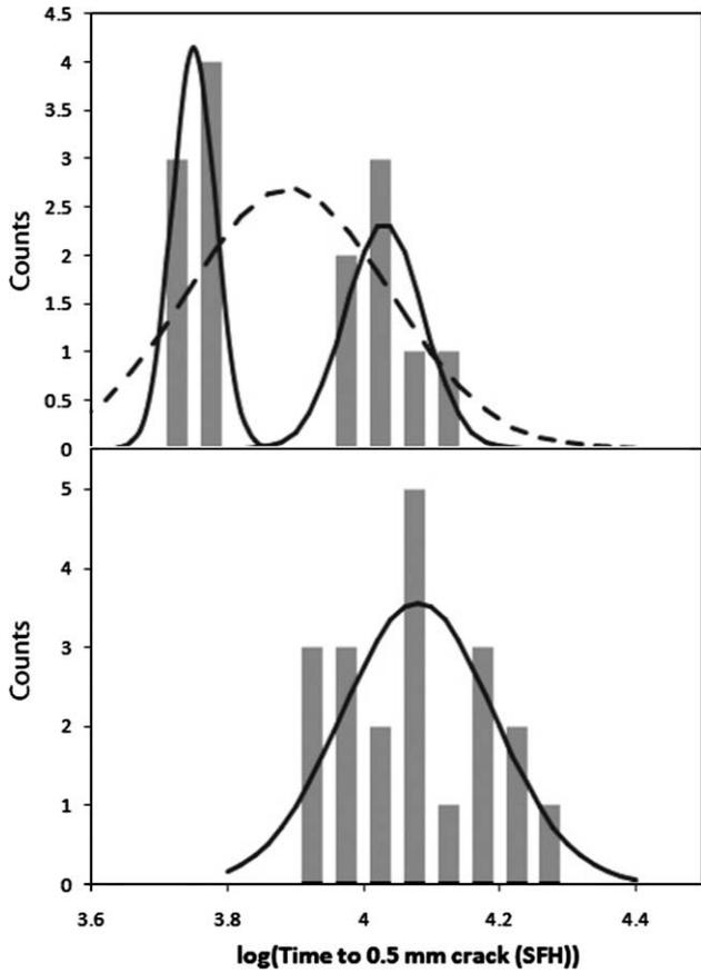
**Fig. 1.** Comparison of the fatigue life distributions for a spectrum with small cycles (M0) (top) and a filtered spectrum (M19) (bottom) [2]. The solid curves represent normal distribution fits to the data. The dashed curve is a normal distribution fit to all of the M0 data, ignoring the bimodal behaviour.
