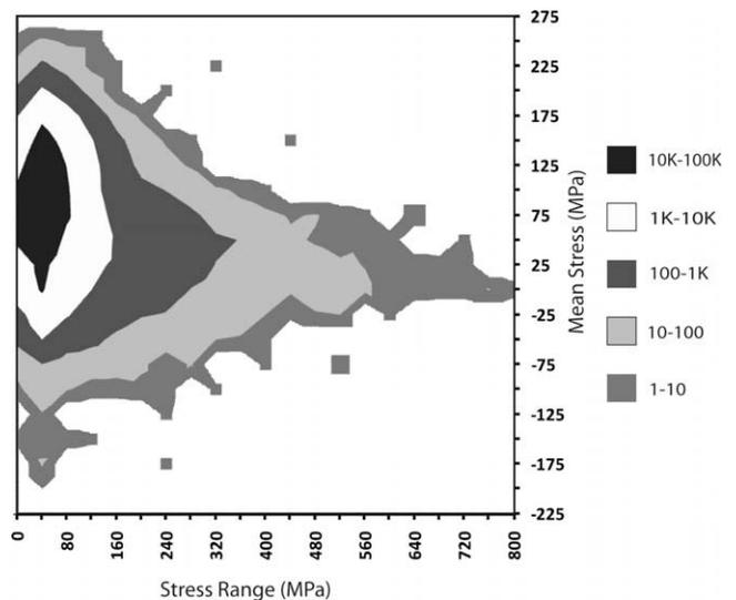
**Fig. 2.** Plot of log(number of cycles) versus mean stress and stress range for rain flow counted base spectrum. The numbers along the X and Y axes represent the lower bound on the bin into which the cycles have been partitioned.
