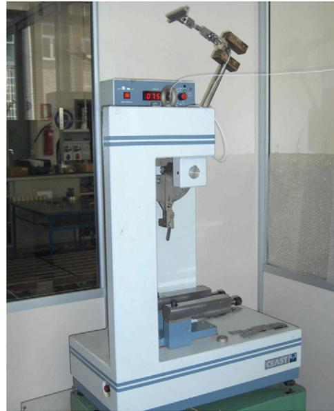
Fig. 1. Instrumented pendulum carrying a specimen.
