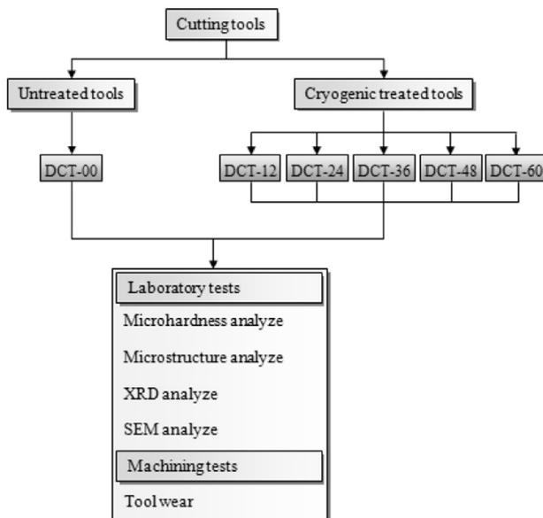
Fig. 1. Flow chart for experimental procedure.
