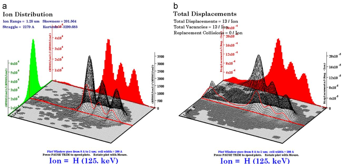
Fig. 1. 3D presentation of (a) hydrogen distribution and (b) defects distribution in silicon:  $E = 175, 150$  and  $125 \text{ keV}$ ; respective doses = 10,000, 10,000 and 15,000 counts; the surface of silicon is on the left hand side of the graph (Note: in this figure 125 keV is indication of the last implant).
