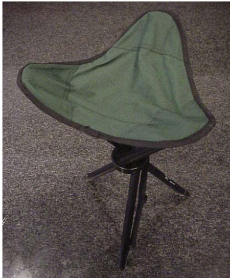
Fig. 1. (a) Support legs and stability arrows for chair legs ranging from elastically averaged to kinematic. (b) Kinematic design principles applied to create a collapsible camping stool as a modern variation of the classic three-legged milking stool.
