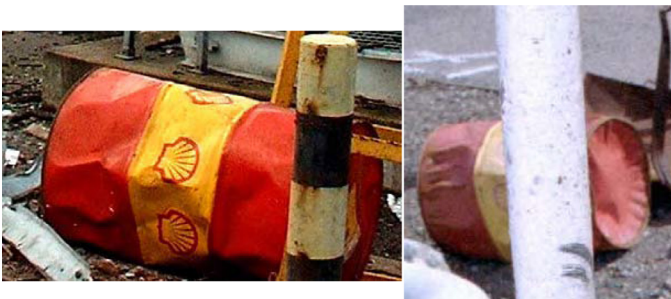
Fig. 2. Typical damaged drums [1].
