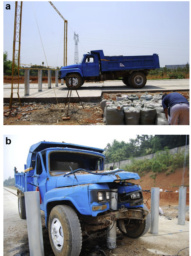
Fig. 2. Truck in the field test: (a) before collision; (b) after collision.
