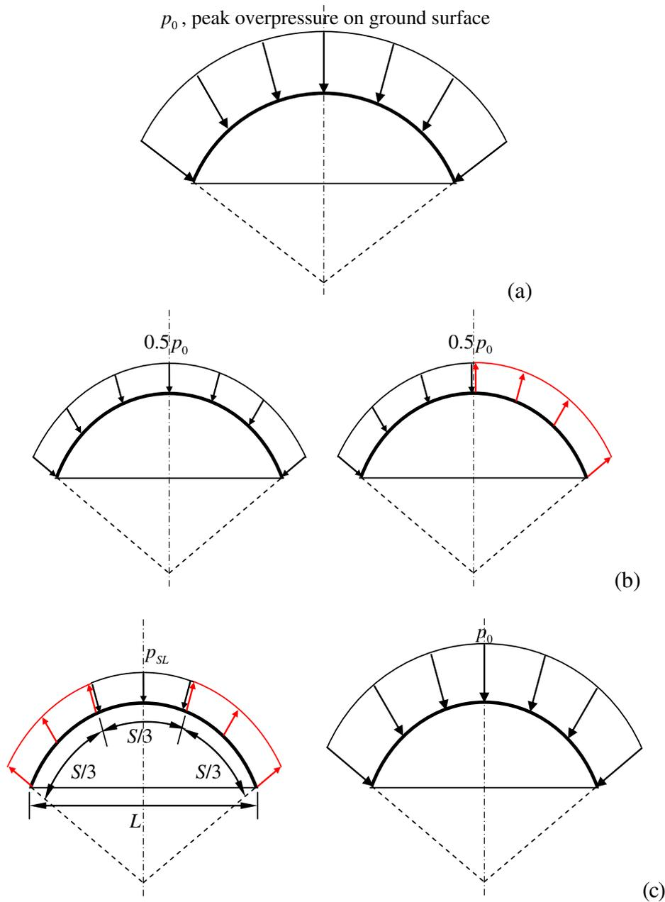
Fig. 1. Recommended idealized loadings for nuclear explosions in (a) compression mode; (b) deflection mode; and (c) compression-bending mode [2].
