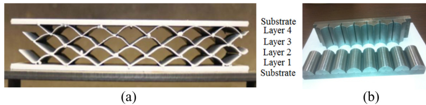
Fig. 1. (a) Corrugated sandwich plate and (b) Die used for making corrugated cores.
