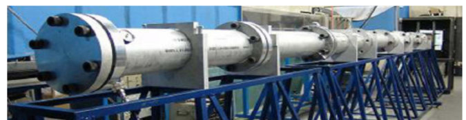
Fig. 2. The shock tube facility [23].
