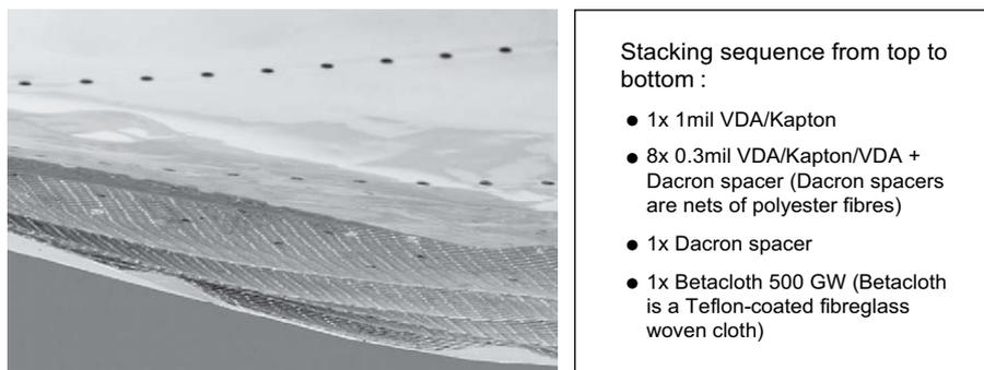
Fig. 1. Configuration of MLI used in the study reported here. The Beta cloth and last Dacron spacer shown above were removed prior to testing since this is not representative of a 'typical' MLI configuration. Kapton is a polyimide film; VDA = vapor deposited aluminum.
