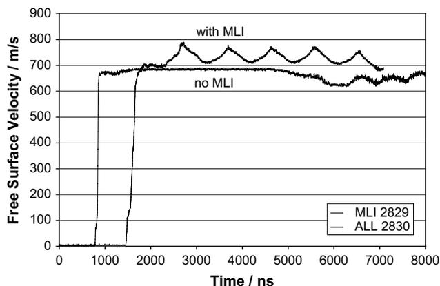
Fig. 2. Preliminary MLI PPI test results. The impact conditions were: 8 mm Al → (0.7 mm MLI) + 3 mm Al. In the case of 'no MLI' an Al-projectile impacts on an Al target. In the other test, the target was covered with MLI on the impacted side.
