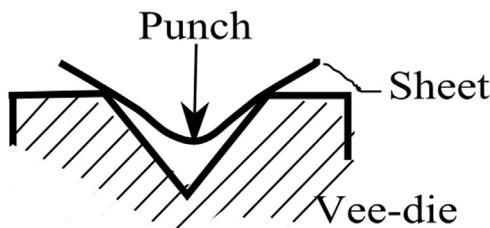
Fig. 1. Schematic of vee-die bending.
