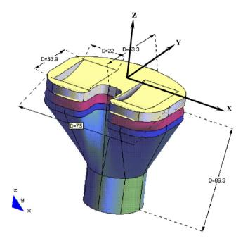
Fig. 2. The configuration and outer dimensions (mm) of the artificial knee joint considered.
