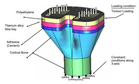
Fig. 3. Assigned material, loading and boundary conditions of FE model.
