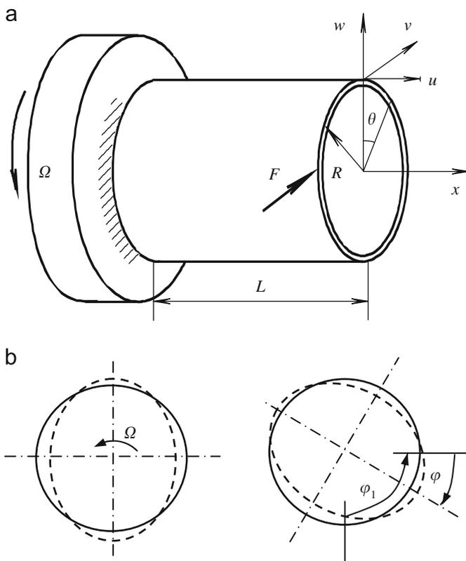
Fig. 1. (a) Coordinate system of a rotating cylindrical shell and (b) precession of vibrating shape of a rotating cylindrical shell.
