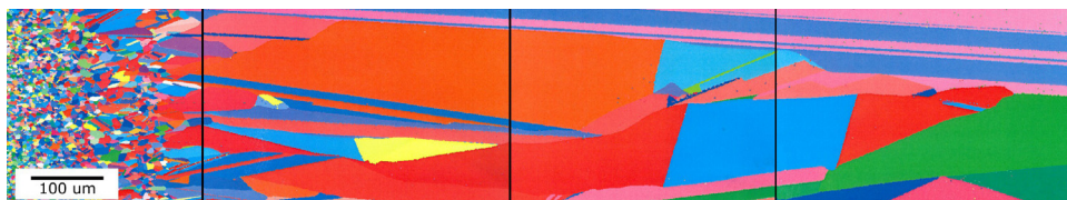
Fig. 1. EBSD image of an electron beam crystallized absorber on glass.
