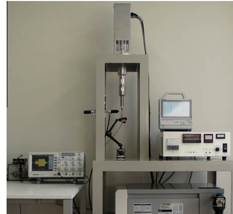
Fig. 3. Ultrasonic fatigue test machine ( f = 19.8 kHz).
