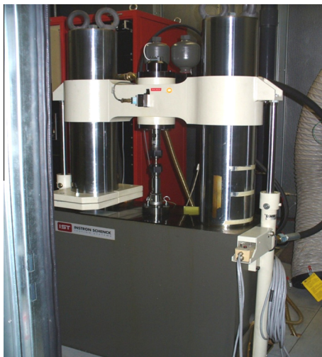
Fig. 2. Servo hydraulic fatigue test machine ( f = 400 Hz).
