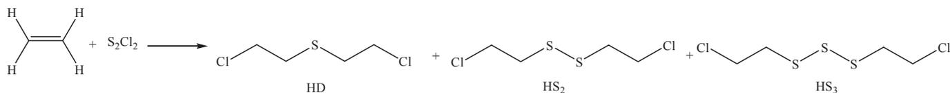
**Scheme 1.** Levinstein process for the production of HD and its two polysulfide analogues.
