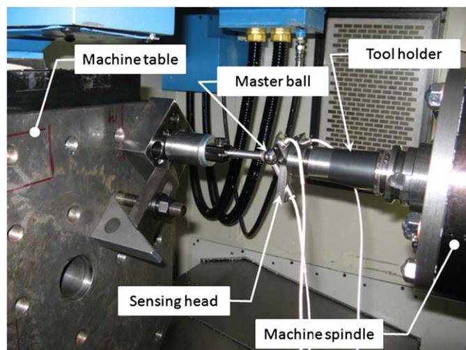
Fig. 1. Functional prototype consisting of a sensing head equipped with three capacitive sensors mounted at the tool holder and a master ball mounted on the machine table.
