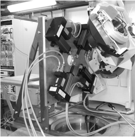
Fig. 1. Uniaxial fatigue machine in DiffAbs beamline.
