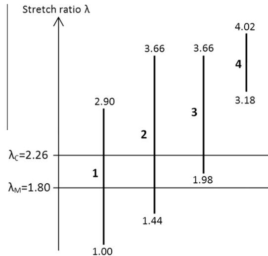
Fig. 2. Minimum and maximum stretch ratios reached during fatigue tests and threshold stretch ratios for crystallization  $\lambda_C$  and melting  $\lambda_M$ . Bold numbers stand for the fatigue tests numbers.
