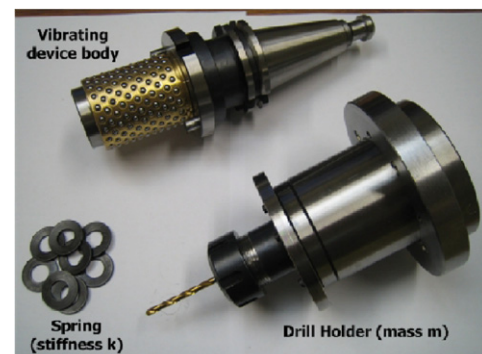
Fig. 1. The self-vibrating drilling head.
