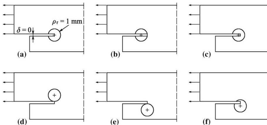
**Fig. 1.** Ambiguity of notch positioning in the FNR approach applied to the weld root of a butt weld joint with backing plate (symmetry half of the model): concentric circle (a), eccentric circle horizontally displaced to different extents (b and c) and eccentric circle vertically displaced to different extents (d, e and f).
