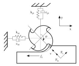
Fig. 1. Mechanical model (down-milling).
