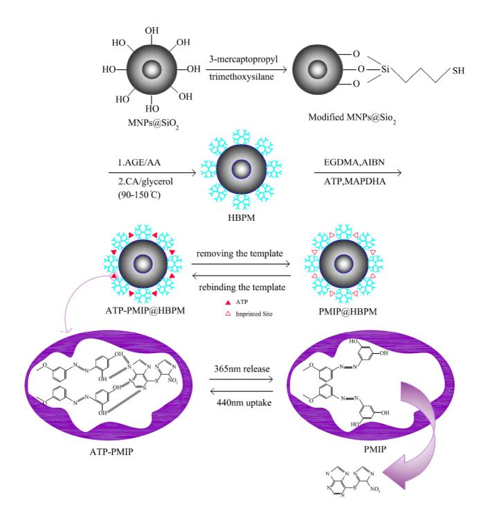
Fig.2. Schematic representation of the PMIP@HBPM process
