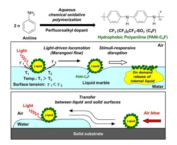
Synthesis of hydrophobic polyanilines as a light-responsive liquid marble stabilizer by aqueous chemical oxidative polymerization
