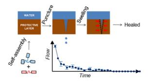
Nitroarylurea-terminated supramolecular polymers that exhibit facile thermal repair and aqueous swelling-induced sealing of defects
