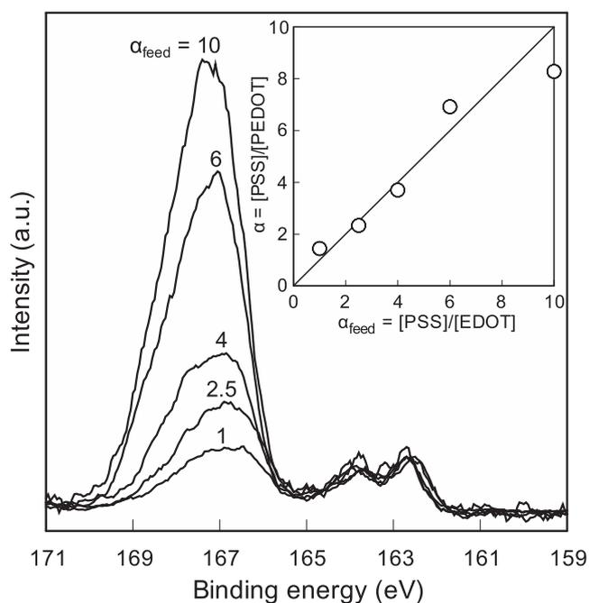
Fig. 1. XPS spectra of PEDOT:PSS with various feed composition ratios ( $\alpha_{\text{feed}}$ ) of PSS repeating unit to EDOT monomer in the energy range of the S 2p signal. Inset: Relation between  $\alpha_{\text{feed}}$  and actual composition ratio ( $\alpha$ ) of repeating units for PSS and PEDOT estimated from the XPS spectra.
