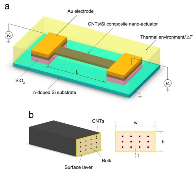
**Fig. 1.** (a) Sketch of CNTs reinforced electrostatic nano-actuator system under thermo-electric loads. (b) Cross section of CNTs reinforced nano-actuator with surface layer.
