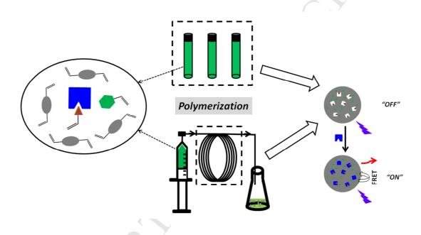
Molecularly imprinted polymer nanoparticles bearing a suitable fluorescence acceptor were synthesized by precipitation polymerization in one-pot as well as in a continuous microfluidic reactor. The imprinted nanoparticles emit strong fluoresce when they bind to an analytical target.
