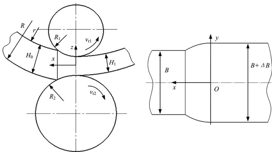
Fig. 1. Schematic illustration of large cylindrical shell rolling.
