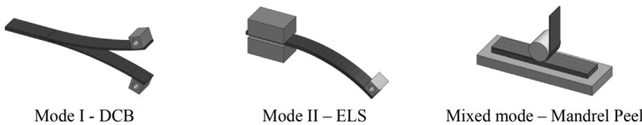
Fig. 1. DCB, ELS, and Mandrel Peel test scheme.
