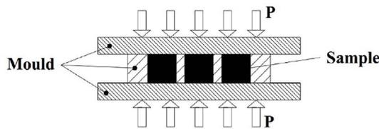
Fig. 1. Sketch of the vulcanisation of isotropic MREs.
