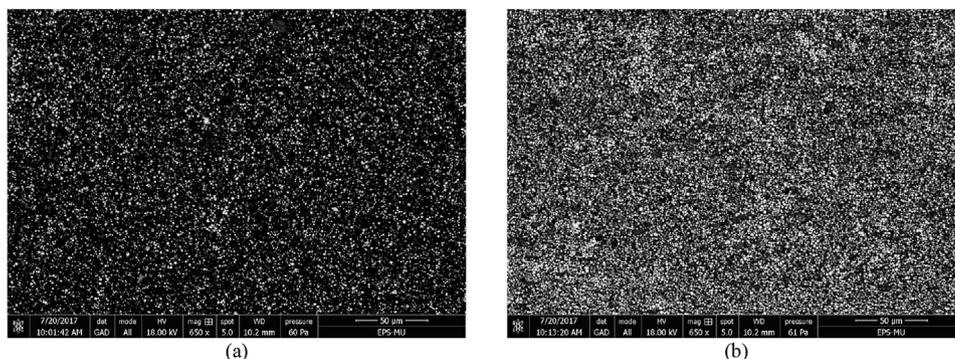
Fig. 2. SEM images of (a) 15% and (b) 30% isotropic MRE samples in low-vacuum conditions and with a voltage acceleration of 18 kV.
