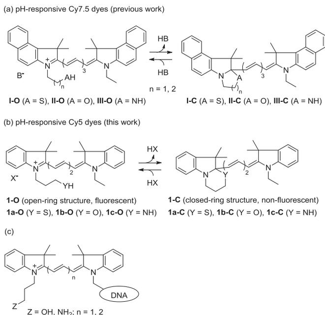
**Fig. 1.** (a) pH-Responsive Cy7.5 dyes (our previous work) and (b) pH-responsive Cy5 dyes (this work). Equilibrium between **1-O** having an open-ring structure and **1-C** having a closed-ring structure. (c) Cy3 and Cy5 derivatives as DNA labeling agents.
