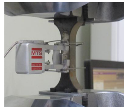
(c) Side view of a specimen on the testing machine
