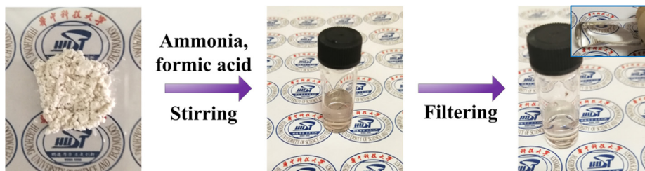
Fig. 1. Schematic preparation process of the reactive silver ink.
