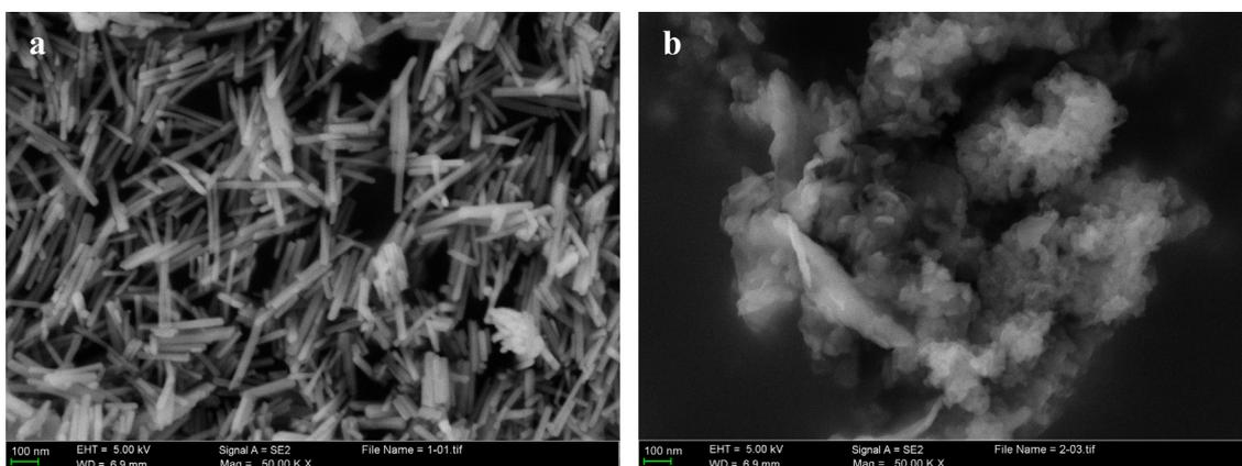
Fig. 2. FE-SEM images of  $\text{ZnWO}_4$  (a) and  $\text{g-C}_3\text{N}_4$  (b).
