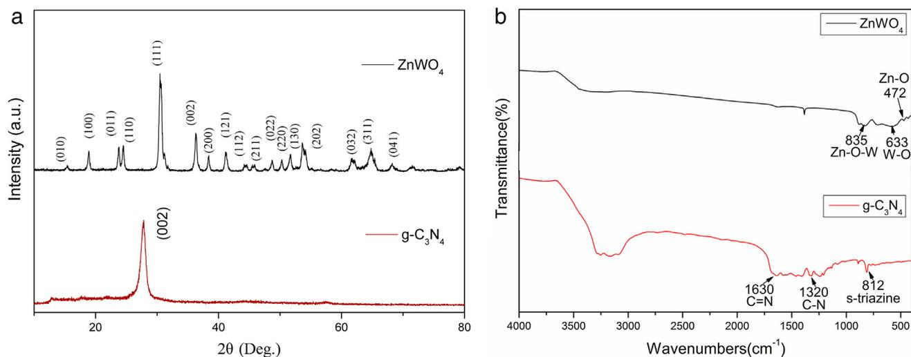
Fig. 1. XRD (a) and FT-IR (b) of  $\text{ZnWO}_4$  and  $\text{g-C}_3\text{N}_4$ .
