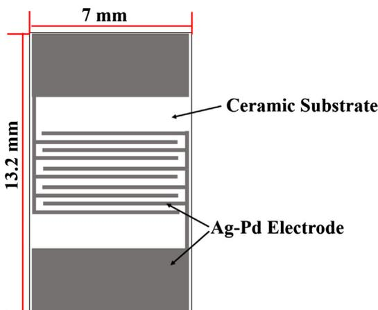
Fig. 1. Schematic diagram of sensor electrode substrates.
